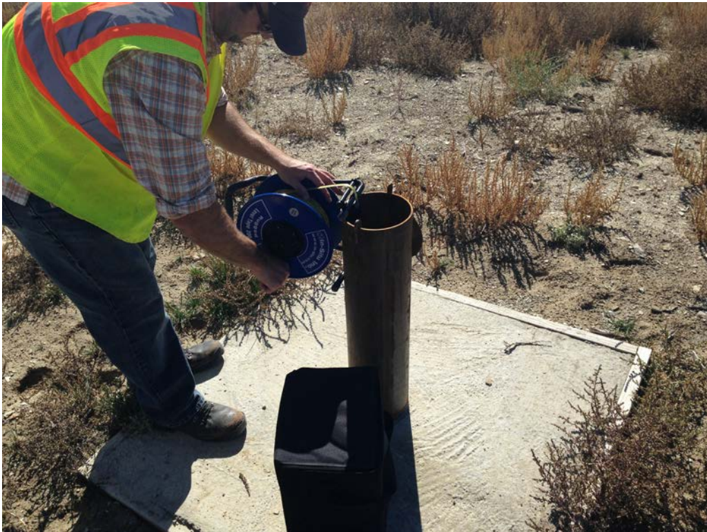
Figure C- 6. Obtaining the Initial Depth to Water Level Measurement at MW-03.
