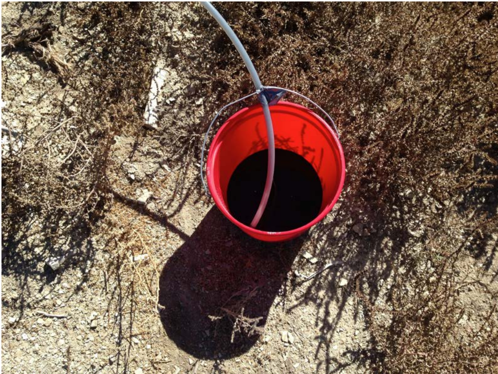
Figure C- 8. View into Graduated Bucket Containing Black Discolored Discharge Water from MW-03.
