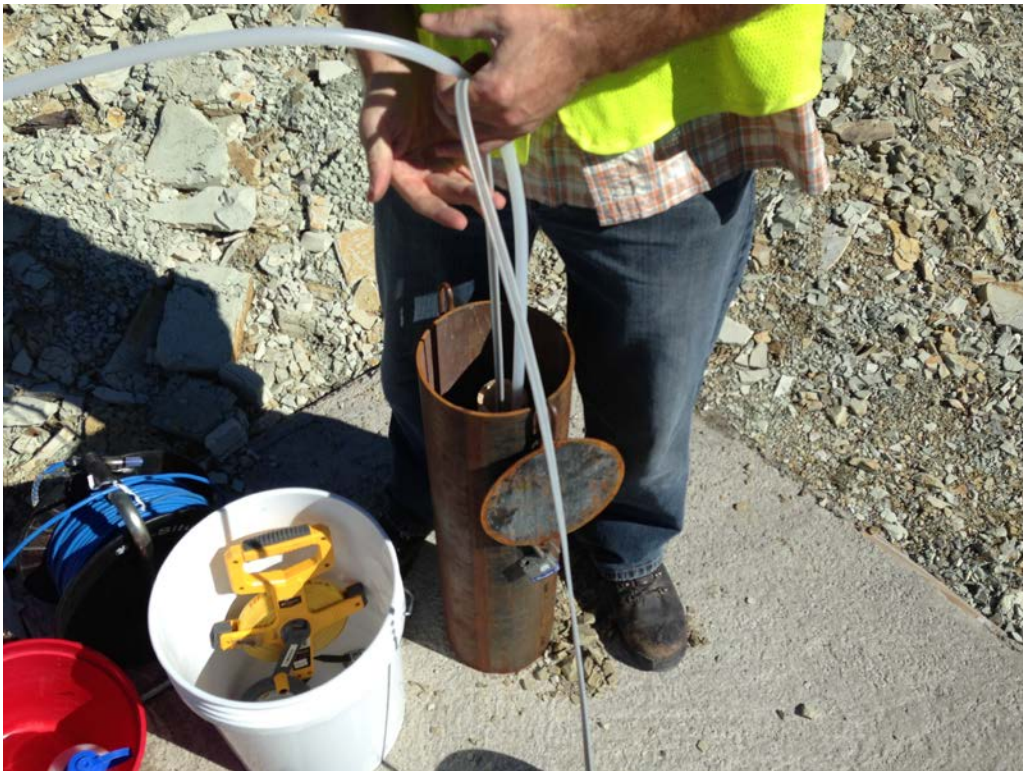
Figure C- 4. View of Pump and discharge tubing being lowered into MW-02.
