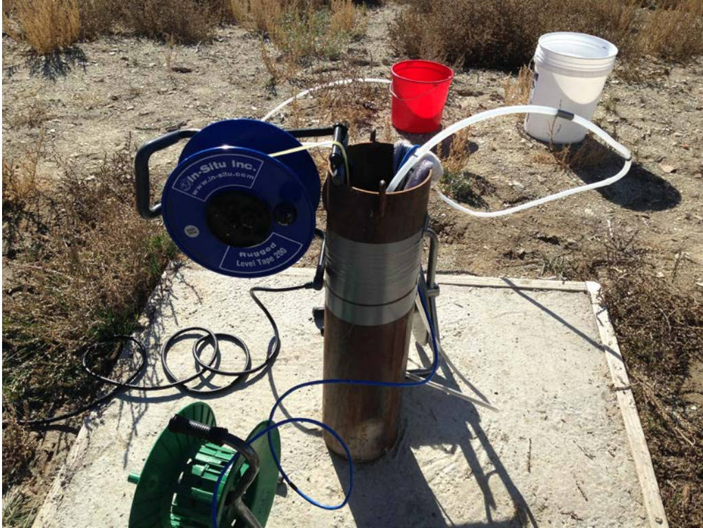
Figure C- 1. View of Aquifer Test Setup at MW-01.
