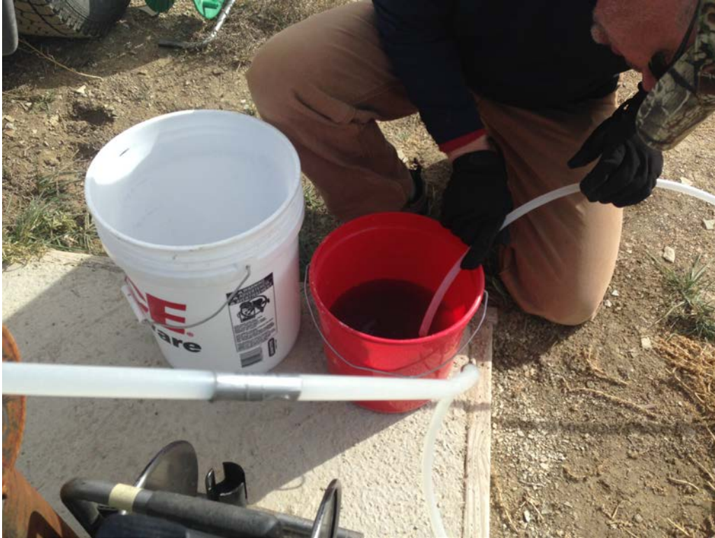
Figure C- 3. View of Dark Gray Discolored Discharge Water Being Measured with a Graduated Bucket. At MW-01
