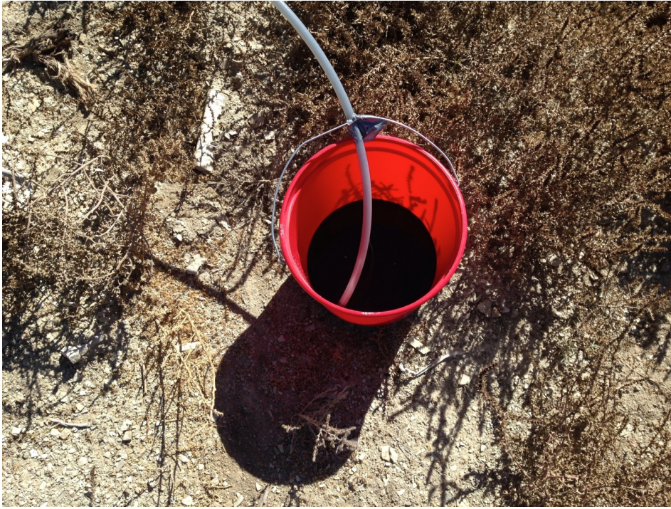
Figure 9-13 View into Graduated Bucket Containing Black Discharge Water from MW-03
