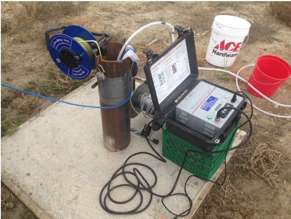
Figure C- 2. Close-up View of Pump Controller (right) and Electronic Water Level Measuring Tape (left) at MW-01.
